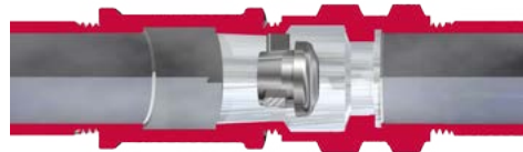
Plug held open by fusible metal alloy.
