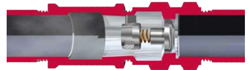
Alloy melts and plug is pushed closed by spring.
