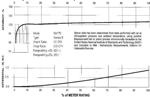
As expected, this curve illustrates the meter accuracy is well within the +/-1% range specified by the ANSI standard for flow rates between 10% and 100% of meter capacity.
