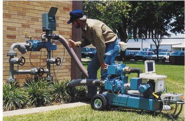
**Above:** Testing a rotary meter with a transfer prover
