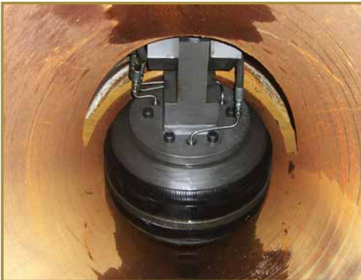
BISEP™ deployed into test pipe
